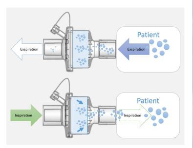
One important parameter for Heat and Moisture Exchanger is the moisture loss. The test method is specified in DIN EN ISO 9360-1. The moisture loss represents the total amount of absolute humidity lost from the HME medium that retains a portion of the patient's expired moisture and heat which should be returned to the respiratory tract during inspiration.
